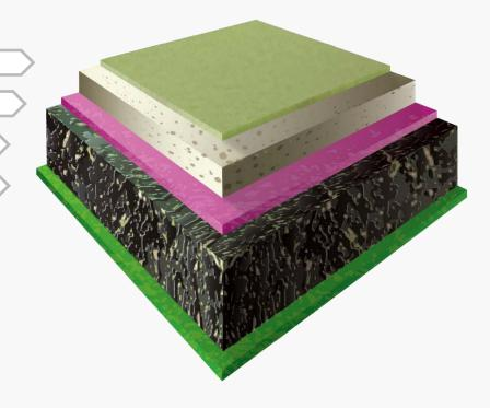
Dynapoint<sup>®</sup> Classic is a resilient, seamless sandwich indoor sports flooring system. Composed of prefabricated recycled rubber mat adhered to the substrate and coated with a minimum 2mm premium polyurethane Wear Coat. Finished with two layers of premium polyurethane matte top coats.
